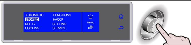
5. Select the type of desired cycle by rotating the knob
