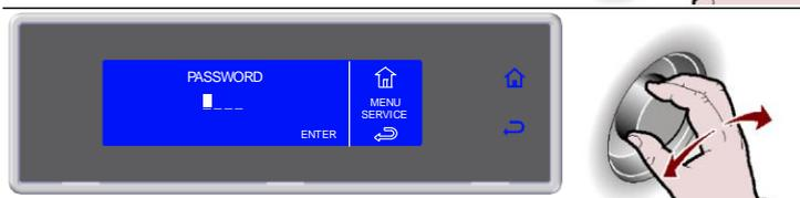
8. Press the knob to confirm and enter section PARAMETERS
