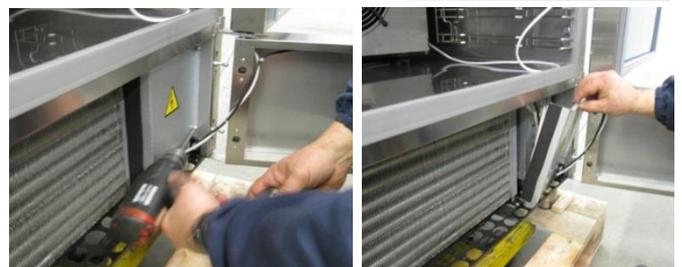
Remove the electrical panel locking screw.
