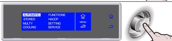
5. Select the type of desired cycle by rotating the knob
