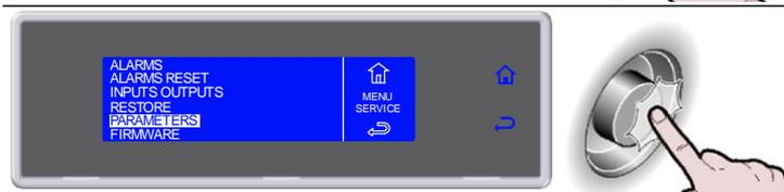
7. Enter the password by turning the knob and press to confirm the value and move to the next one until ENTER is selected
