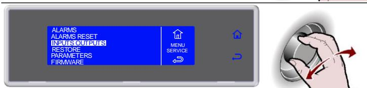
6. Press the knob to view the list INPUTS OUTPUTS
