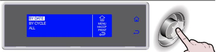
9. Enter the data by turning the knob and press to confirm the value and move to the next one until ENTER is selected
