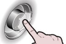
9. Enter the data by turning the knob and press to confirm the value and move to the next one until ENTER is selected
