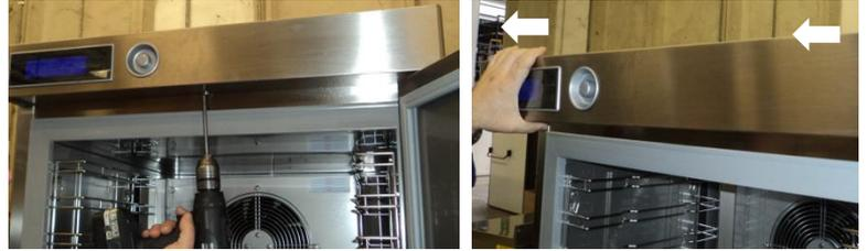
Undo the guard screws and remove the cover to access to the video card and to the encoder.
