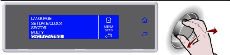
6. Press the knob to enter section CYCLE CONTROL
