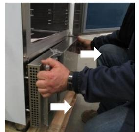
Remove the closing panel screws.
