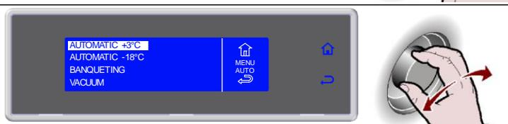
6. Press the knob to enter into the selected type of cycle
