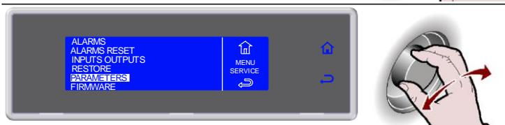
6. Press the knob to enter section PARAMETERS
