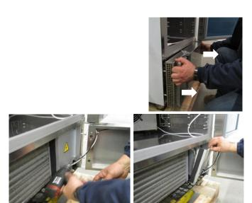
Remove the electrical panel locking screw. Move the electrical panel box along the slide.
